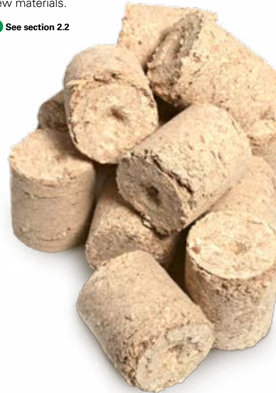
Wood pellets – a form of biomass energy used from domestic boilers to large power plants.
