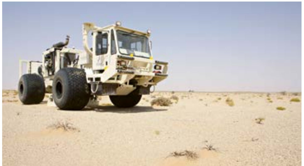
Digitizing the search for gas – vibrator trucks carry out seismic operations for BP in the desert of Oman.
