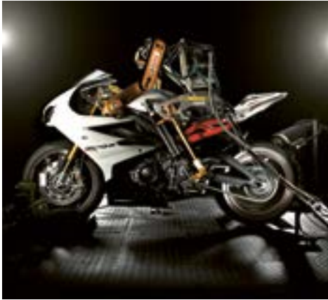
A robot rides a motorcycle to test Castrol lubricants – robots are used to improve test repeatability and safety.
