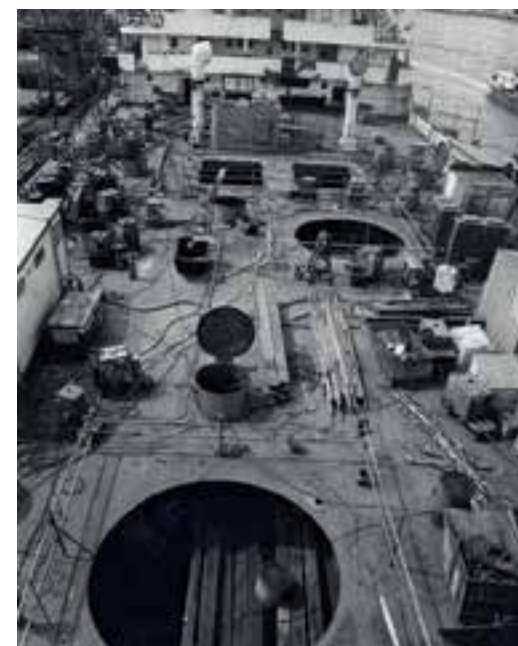
Holes are cut in Kiwi's deck to accommodate retractable propellers for close docking purposes.
