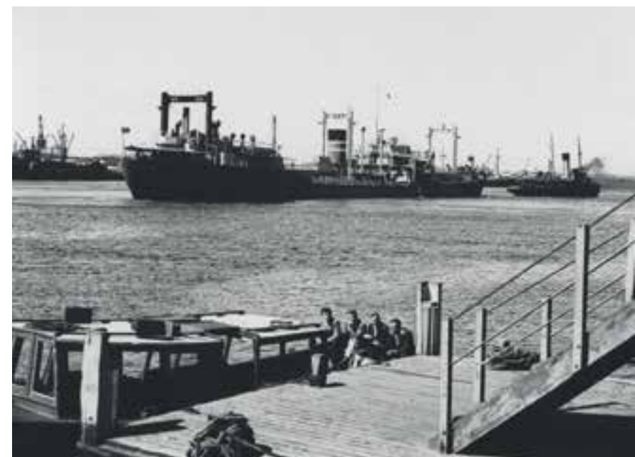
British Cavalier was originally launched as Empire Cavalier in 1942 for the Ministry of War Transport. She was fitted with a dummy funnel in the middle of the vessel to disguise that she was a tanker – and a very attractive target for U-boats. She was managed by BTC for part of the war and purchased in 1945, with the dummy funnel retained for some time afterwards. Later images show her with a single funnel aft – up to her scrapping in 1959.
