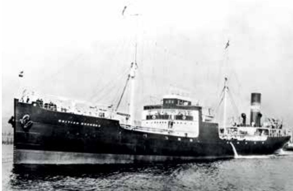
British Duchess – 9,000 dwt steam-engine tanker – matched the new combustion engine of the motorship British Renown in a race from the Mediterranean to the UK. She was sold in 1952 after 28 years' service.
