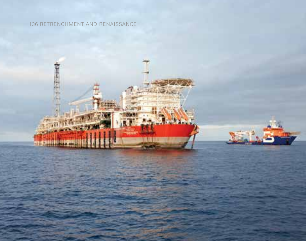
Left and below: Greater Plutonio floating production storage and offloading facility located in the South Atlantic Ocean off the coast of Angola.
