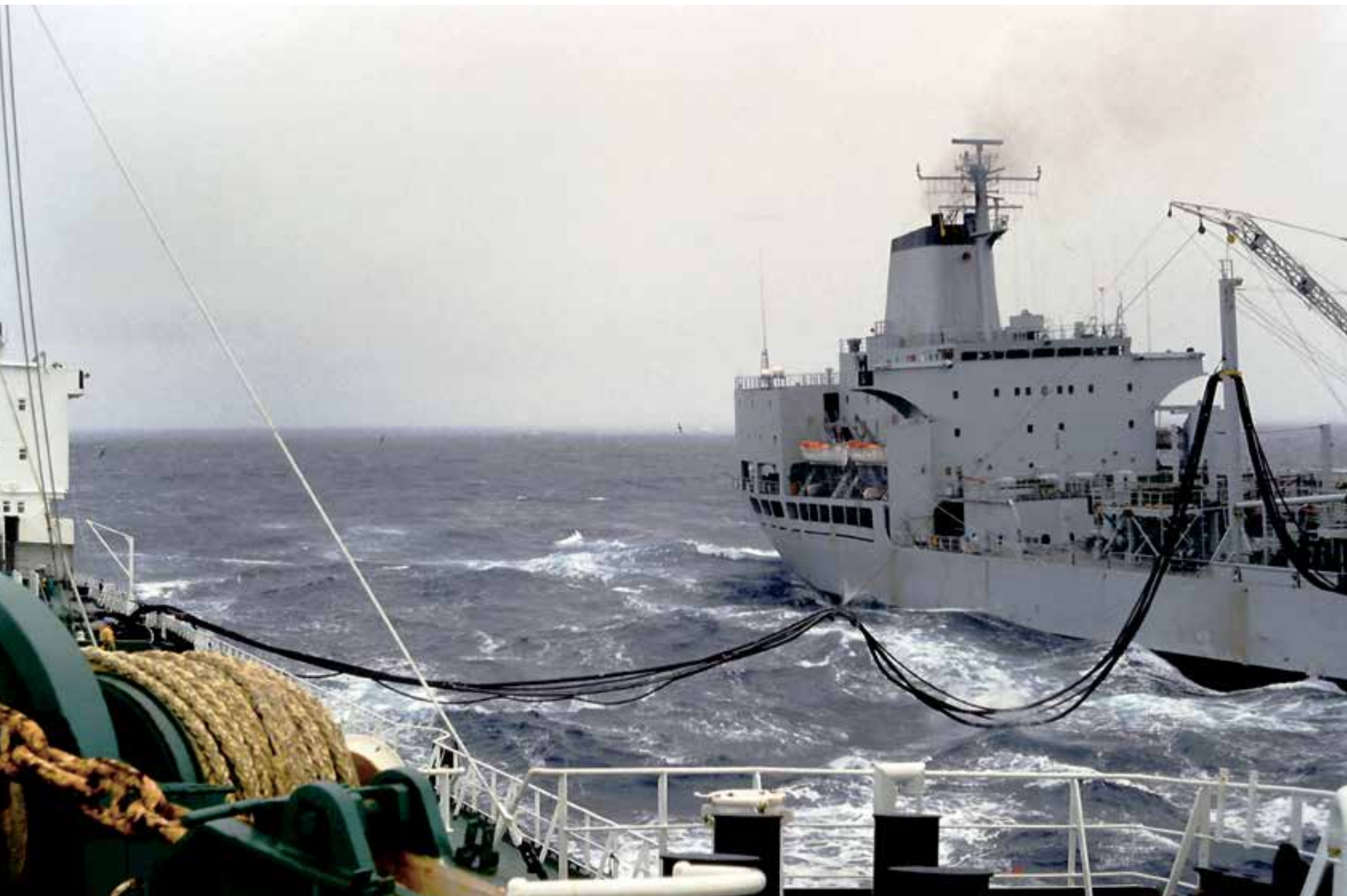
Ship-to-ship refuelling on a relatively calm day in the South Atlantic.
