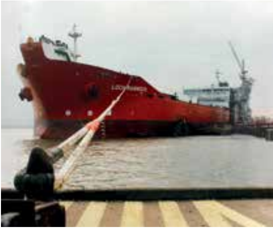
Loch Rannoch – a dynamically positioned shuttle tanker – developed during the 1990s as part of the Schiehallion field FPSO.
