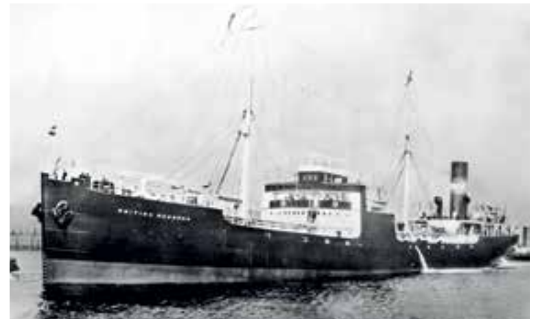
Above: British Duchess – 9,000 dwt – was one of more than sixty tankers built for BTC in the 1920s. Her fairly rudimentary layout included all aft accommodation for the crew. She served in the fleet for 28 years.
