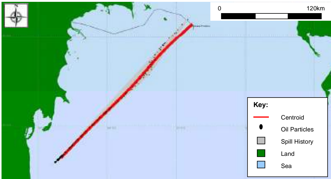
Figure 20 Spill history for Scenario 1A.10 showing the trajectory of the 24 hour oil spill. The grey area indicates the area most likely to be affected by oil sheening.
