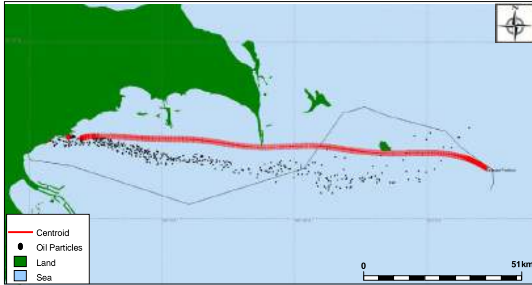
Figure 3 Spill history for Scenario 1A.15 showing the trajectory of the 24 hour oil spill
