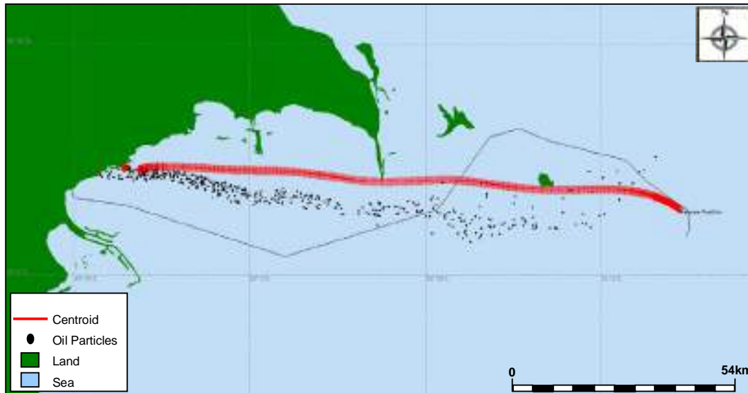
Figure 1 Spill history for Scenario 1A.13 showing the trajectory of the 24 hour oil spill
