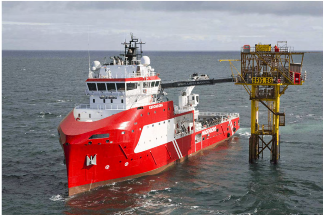
Figure 5.16: Example of a walk-to-work maintenance vessel
