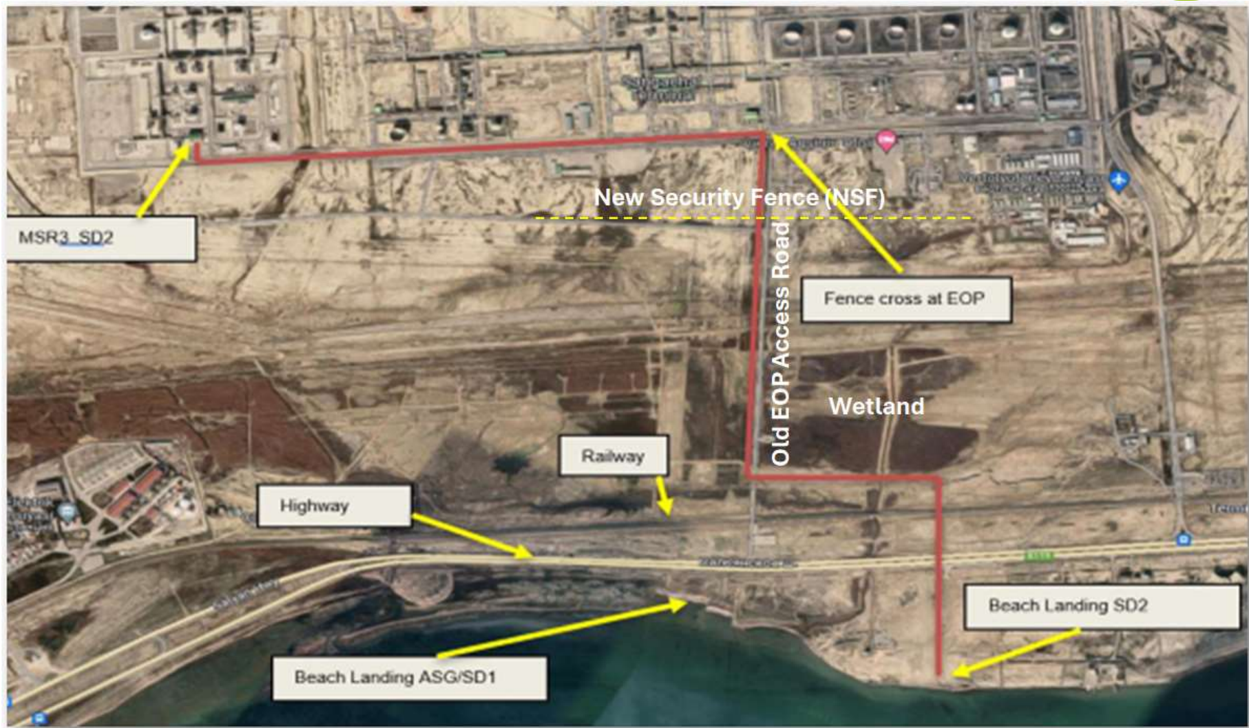
Figure 5.13: Proposed onshore section of Sangachal to SDC PFOC route (only section from the landfall in Sangachal Bay to the new security fence within scope)
