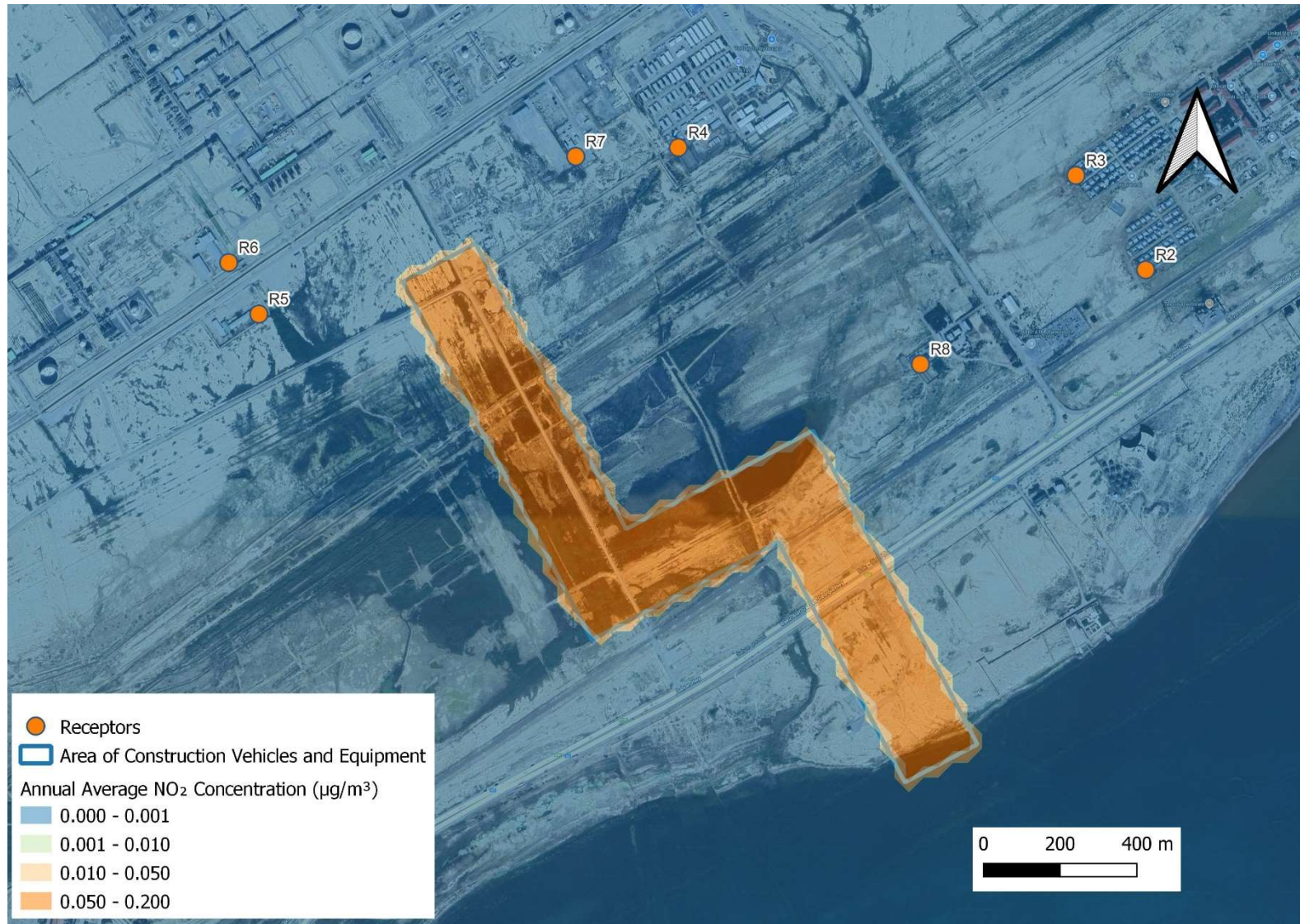
Figure D.5: Contour plot annual average NO 2 concentrations - onshore PFOC route (using 2020 meteorological dataset)
