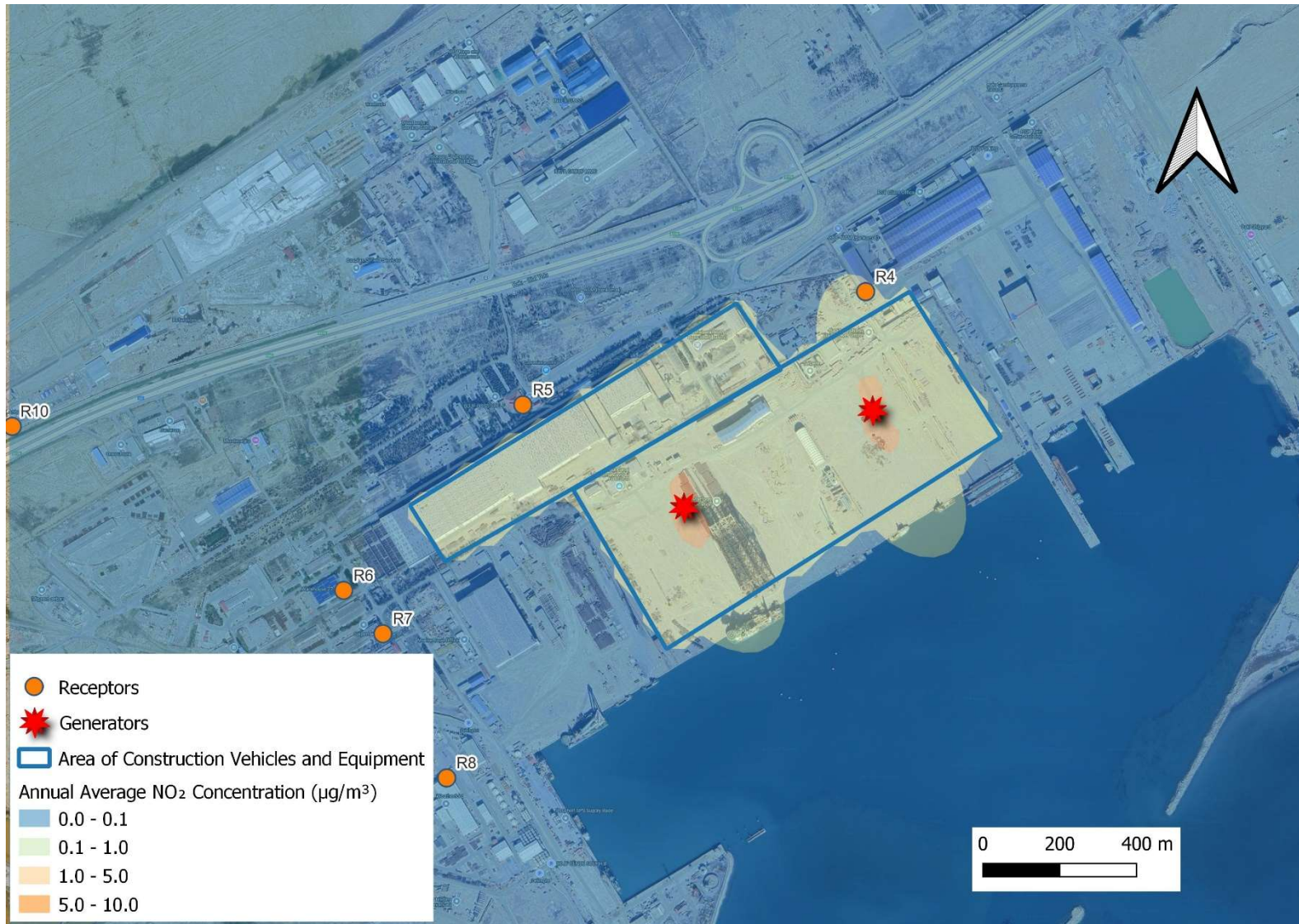
Figure D.1: Contour plot annual average NO 2 concentrations - BDJF yard (using 2021 meteorological dataset)
