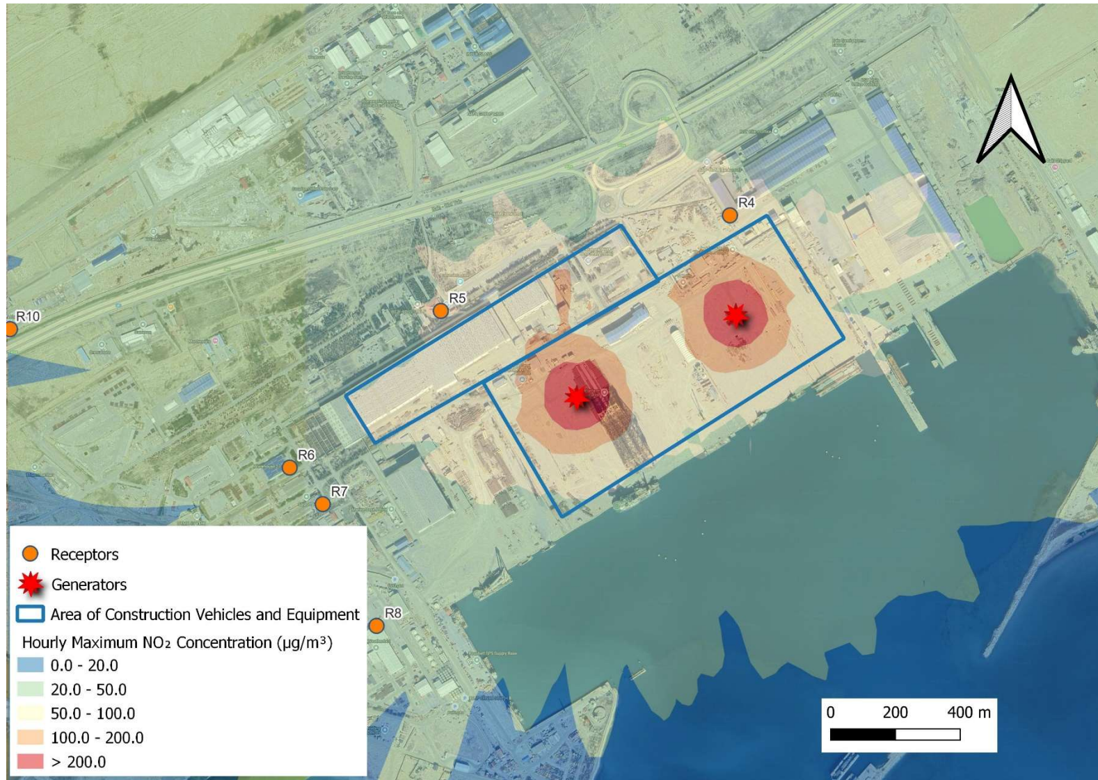
Figure D.2: Contour plot hourly maximum NO 2 concentrations - BDJF yard (using 2021 meteorological dataset)
