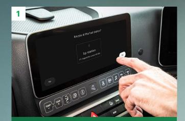
Once at the service station, the driver uses the In-Truck Connect app to locate and connect to the station via GPS
