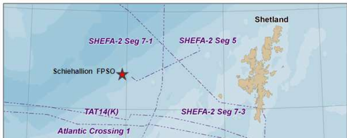
Figure 4-3 Cables in the area of the Schiehallion and Loyal fields. (Source: KISCA, 2010).
